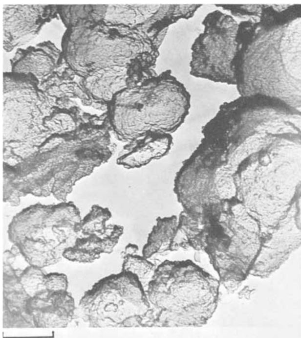
Fig. 3. Electron micrograph of a carbon replica of PbO 2 from oxide A after formation on 7% antimonial lead grids. These agglomerates appear to be true spherulites of small sessile crystals overgrown on spikes of larger crystals. Marker equals approximately 1 \mu .
