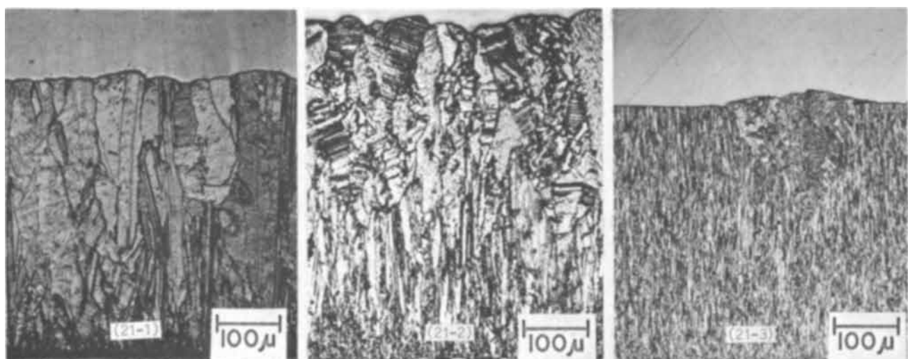
Fig. 21. Effect of periodic current reversal (PR) on the structure of copper deposits from a sulfate bath (Cu2-H3): (21-1) 30°C, 2 A/dm 2 , continuous current; (21-2) 20°C, 4 A/dm 2 , continuous current; (21-3) 30°C, 4 A/dm 2 , PR, 5 sec cathodic, 2 sec anodic.
