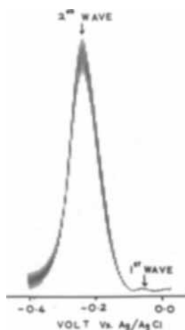
Fig. 1d. Rapid a-c polarogram of antimony(III) in \text{NaClO}_4/\text{HClO}_4 .
