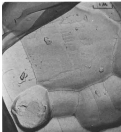
Fig. 6. \beta - \text{Ca}_2\text{P}_2\text{O}_7 , prepared by heating \text{CaHPO}_4 + \text{Sb}_2\text{O}_3
