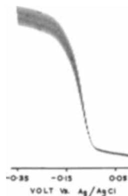
Fig. 4a. D-C polarogram of the antimony(III)- \text{NaClO}_4/\text{HClO}_4/\text{NaI}/\text{NaF} system at high fluoride concentrations.
