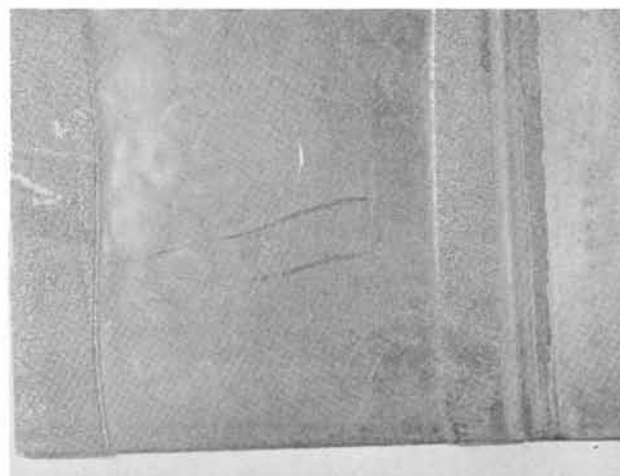
Deposit Produced in Beta-Naphthol Bath (only center portion of sample was heated)
