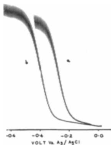
Fig. 3a and b. Effect of added fluoride on the d-c antimony(III)- \text{NaClO}_4/\text{HClO}_4/\text{NaF} polarogram. Figure 3b has a higher concentration of fluoride than Fig. 3a and the negative shift in E_{1/2} due to fluoride complexing can be seen.
