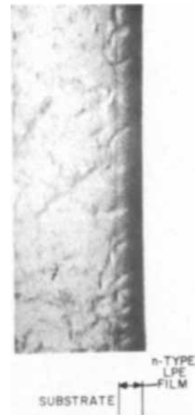
Fig. 5. CF-XRT of GaP substrate — single LPE film profile ( \sim 90\times ).
