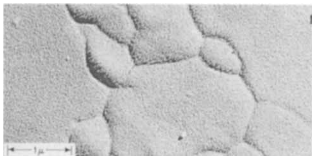
Fig. 1. Electron micrograph of a 0.5\mu evaporated AgBr layer
