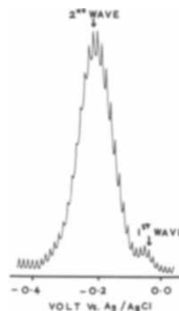
Fig. 1b. Conventional a-c polarogram of antimony(III) in \text{NaClO}_4/\text{HClO}_4 .
