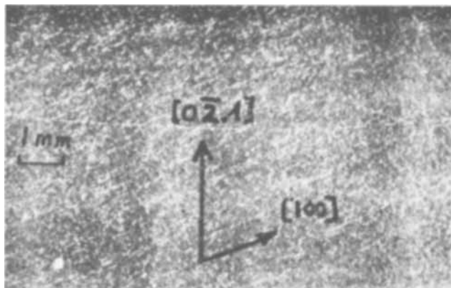
Fig. 1. X-ray surface topography of the sapphire substrate after H 2 etching at 1300°C.
