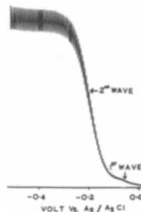
Fig. 1c. Rapid d-c polarogram of antimony(III) in \text{NaClO}_4/\text{HClO}_4 .
