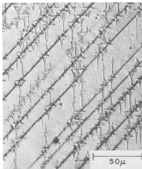
Fig. 3. Aluminum single crystal anodized at 30V and extended 11%. Cracks in coating formed along some of slip plane traces. In addition short circumferential cracks can be observed where buckling has occurred.
