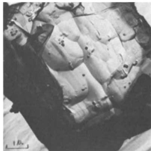
Fig. 10. \text{Ca}_5(\text{PO}_4)_3\text{F} , prepared by heating \text{CaHPO}_4 + \text{CaF}_2
