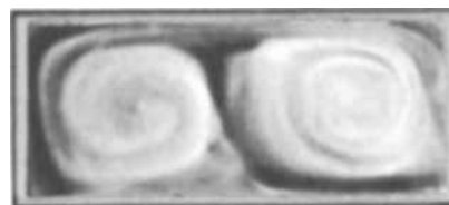
Fig. 2. Streamline pattern above the nonheated susceptor ( T_s \approx 20^\circ\text{C} ) with water-cooling around the tube (wall temperature approximately 10^\circ\text{C} ). Convective flow is visible under the influence of a small vertical temperature gradient. Rotation speed: about 1 rps.
