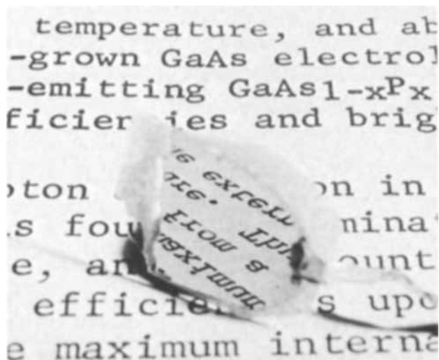
Fig. 3. Reflection from exposed surface of \text{GaAs}_{0.5}\text{P}_{0.5} n-type layer, 5\mu thick, after electrolytic removal of thick p-type GaAs substrate.
