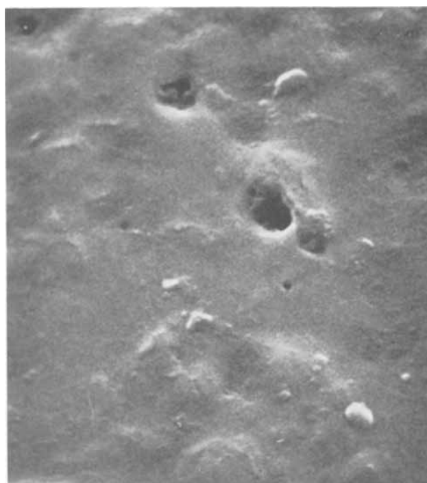
Fig. 13. Uneven growth of anodic oxide films in potassium chromate solution, X 10,000.
