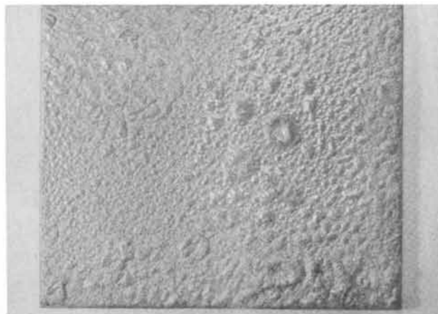
Deposit Produced in Peptone-Resorcinol Bath
