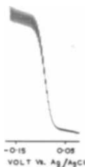
Fig. 2a. Rapid d-c polarogram of antimony(III) in \text{NaClO}_4/\text{HClO}_4/\text{NaI} .
