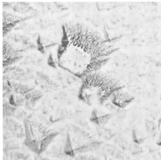
Fig. 4b. Copper deposited from the same electrolyte using the same periodic reverse current cycle as in Fig. 4a. Magnification, 400X.
