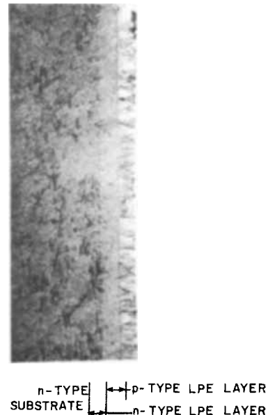
Fig. 6. CF-XRT of GaP substrate — double LPE film profile ( \sim 75\times ).
