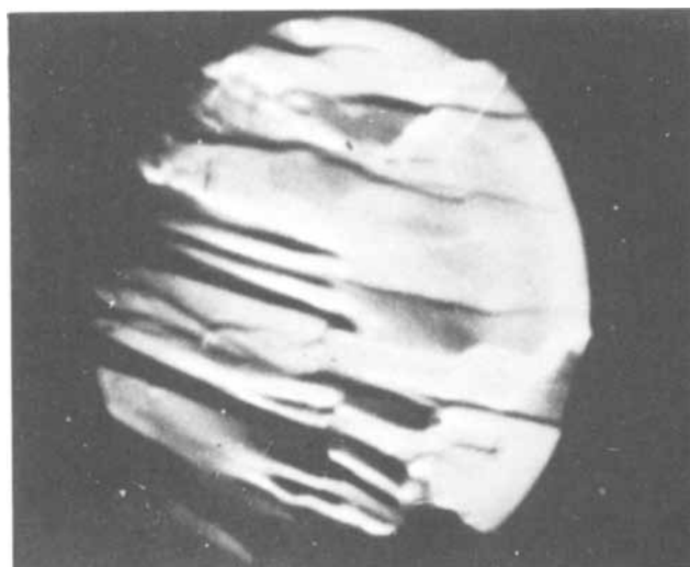
Fig. 6b. X-ray surface topography of the \text{Si-Al}_2\text{O}_3 interface
