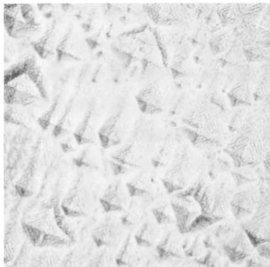
Fig. 4a. Copper deposited from 0.5M \text{CuSO}_4 -0.5M \text{H}_2\text{SO}_4 at 20 \text{mA}/\text{cm}^2 using periodic reverse current cycle of 45 sec direct and 15 sec reverse. Magnification, 400X.
