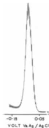
Fig. 2b. Rapid a-c polarogram of antimony(III) in \text{NaClO}_4/\text{HClO}_4/\text{NaI} .
