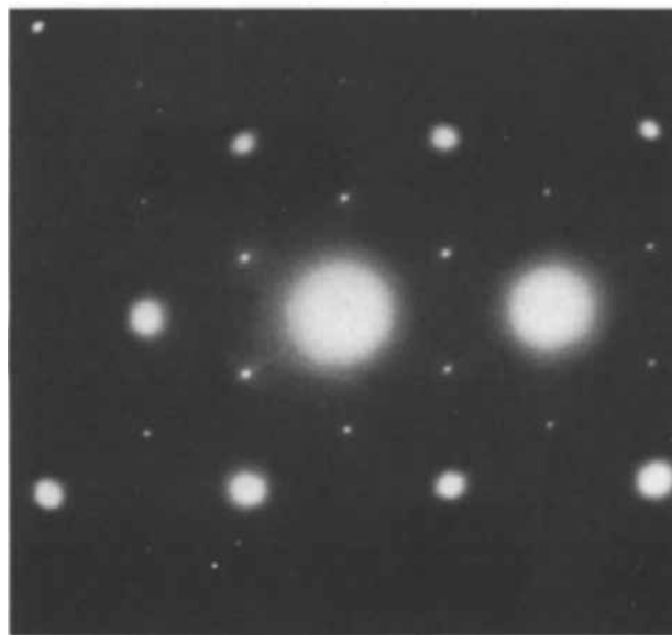
Fig. 2. Transmission electron diffraction pattern of gold deposit on {111} copper single crystal.
